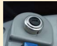
Easy-access, easy-turn ignition with rubber boots for protection against moisture and freezing
