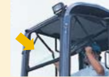
Front window features gas damper cylinders for smooth and easy opening.
