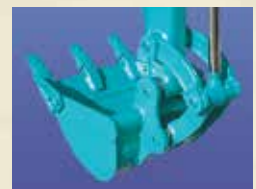
Link pin with locking pin/cast steel idler link
