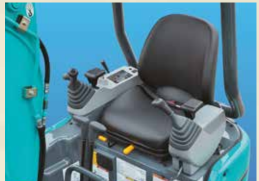
Three-pillar canopy compliant with ROPS and FOPS level 2
